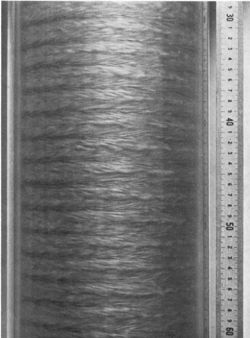
FIGURE 5. Centre section of column of turbulent axisymmetric Taylor vortices in water at T = 3800T_c , \lambda = 3.395 . In narrow gap after a steady acceleration experiment. The equally spaced horizontal lines at which the flow converges are the sinks. The sources are diffuse. Each ring represents a vortex pair.
